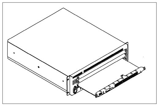
Figure 7. Inserting a Module in the Expansion Unit
